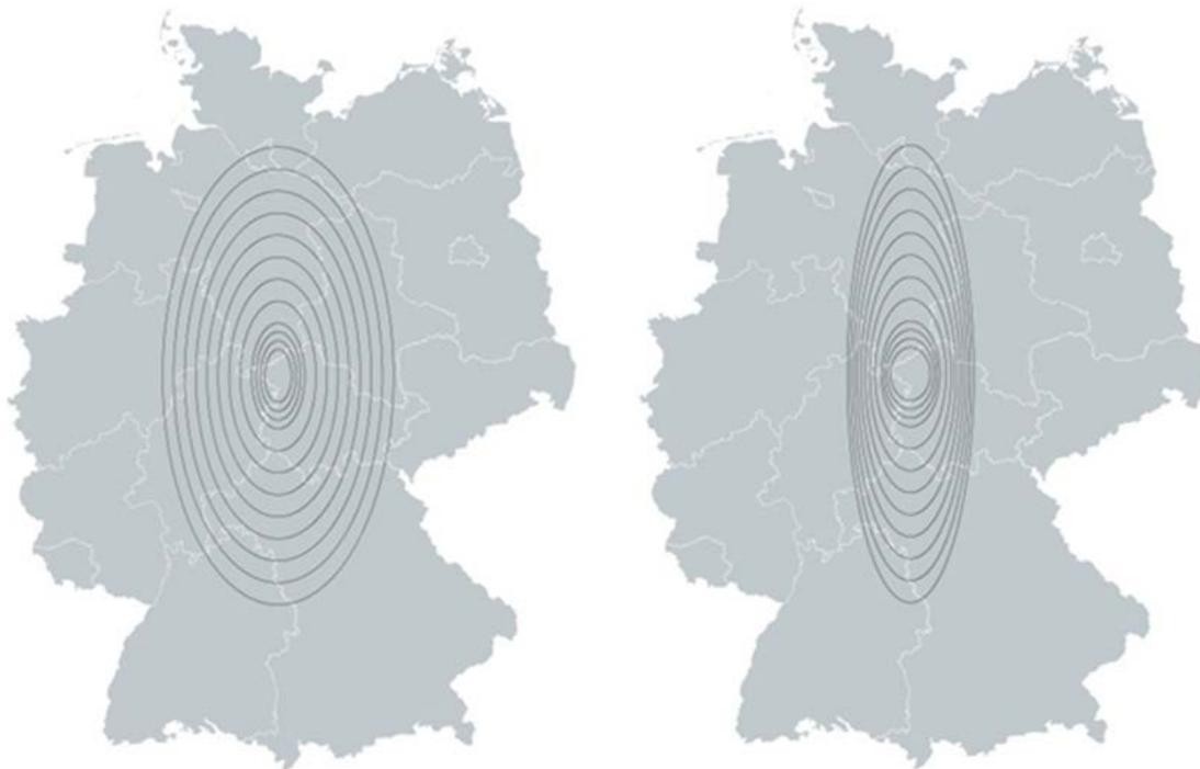
The geometric construction of the ellipses distinguishes between two cases (see Figure 1). In the first case an ellipse is used – as previously – whose minor axis (horizontal axis) measures half of the main axis (perpendicular axis) (2:1 ellipse). This is used for alternating current projects and for direct current projects for which priority is not given by law to underground cabling (currently BBPIG Project 2, Ultranet).
